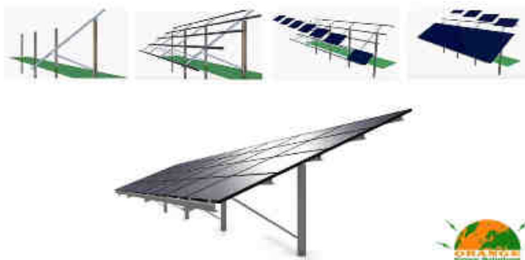
Figur 8: Installation of solcellepaneler
